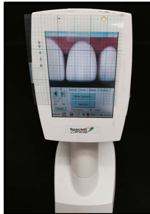
Figure 22. Spectro Shade Spectrophotometer with Grid Attached and Image of the Typodont.
